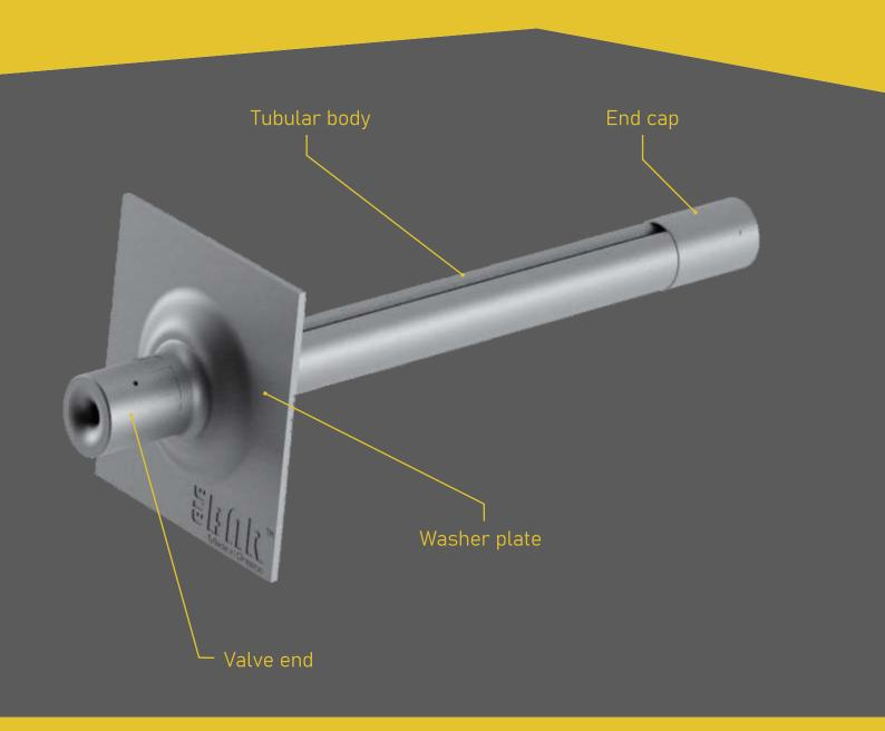
$\mathsf{ELEBOLT}^\mathsf{m}$  is a friction stabilizer that is activated by swelling its tubular steel body after the bolt has been inserted in the borehole. Swelling is achieved by injection of high pressure water in the bolt. The swelling action brings the tubular steel body in true and tight contact to the borehole walls thus exerting radial forces to the surrounding rock/strata.
