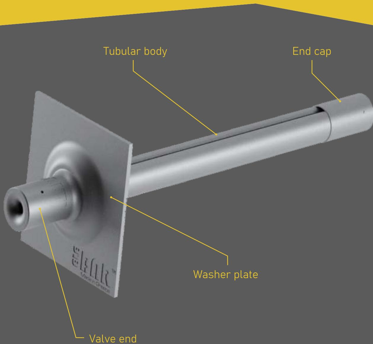
ELEBOLT™ is a friction stabilizer that is activated by swelling its tubular steel body after the bolt has been inserted in the borehole. Swelling is achieved by injection of high pressure water in the bolt. The swelling action brings the tubular steel body in true and tight contact to the borehole walls thus exerting radial forces to the surrounding rock/strata.
