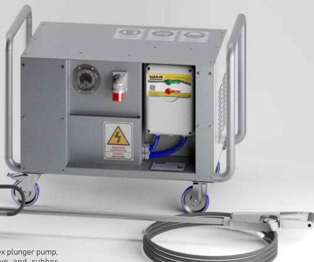
The unit is assembled with a triplex plunger pump, bypass valve, non-return valve and rubber coupler and is equipped with inlet water filter and manometer for the inspection of the outlet pressure.
